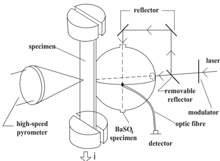
Fig. 1. Schematic of pulse-heating experiments using strip specimens and an integrating sphere.
